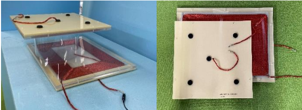
Fig. 21 Measurement scene (Misalignment \Delta X=75 , \Delta Y=100 mm)
